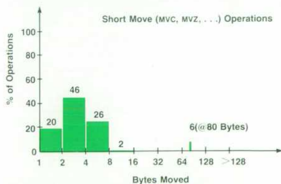
Fig. 3. Storage-to-storage moves were found to move only a few bytes in most cases.
