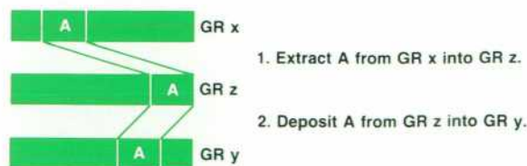
Fig. 7. Movement of an arbitrary field using extract and deposit instructions.
