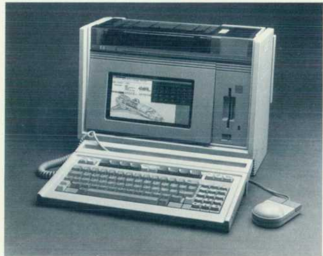
Fig. 2. HP's Integral Personal Computer 2 is a powerful multi-tasking computer system in a 25-lb transportable package. Designed for technical professionals, it features a built-in printer, display, disc drive, and HP-IB interface and the HP-UX operating system, HP's version of AT&T Bell Laboratories' UNIX TM operating system.
