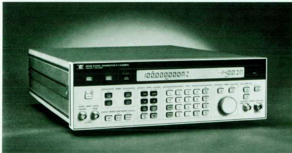
Fig. 1. The HP 8642A/B Signal Generator uses new low-noise oscillator designs with high-Q surface-acoustic-wave (SAW) resonators to improve spectral purity over cavity-tuned generators. Its frequency range is 100 kHz to 1057.5 MHz (A model) or 2115 MHz (B model). High accuracy, wide output power range, and broad modulation capabilities make it suitable for the most stringent receiver tests.
