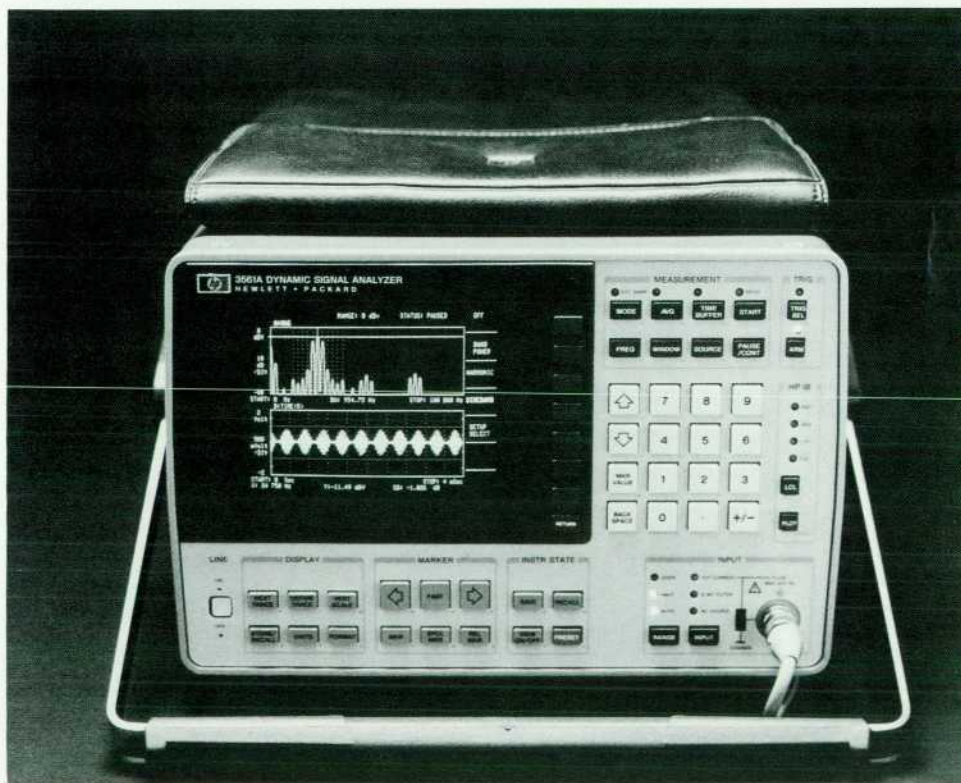
Fig. 1. The HP 3561A Dynamic Signal Analyzer combines high-performance hardware and versatile menu-driven software in a portable package for measurement and analysis of low-frequency waveforms in electronic, acoustic, and vibration applications. Besides spectral analysis, the HP 3561A can perform network measurements and time domain waveform recording.
