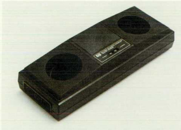
Fig. 1. The HP 82168A Acoustic Coupler can be used to connect any current HP-IL controller such as the HP-75 Portable Computer to a telephone line for transmission of data and programs to another controller or central computer system.
