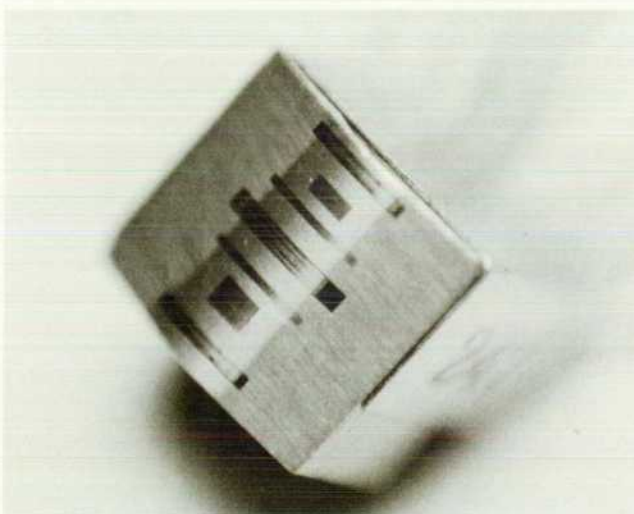
Fig. 3. A common read-after-write head design locates the read and write gaps on opposite sides of the head's crown. The head used in the HP-75 has these gaps located on the crown as shown.
