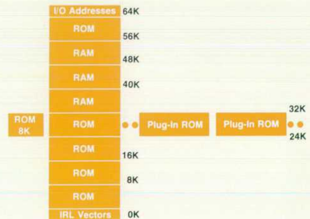
Fig. 3. Memory organization in the HP-75 Portable Computer.
