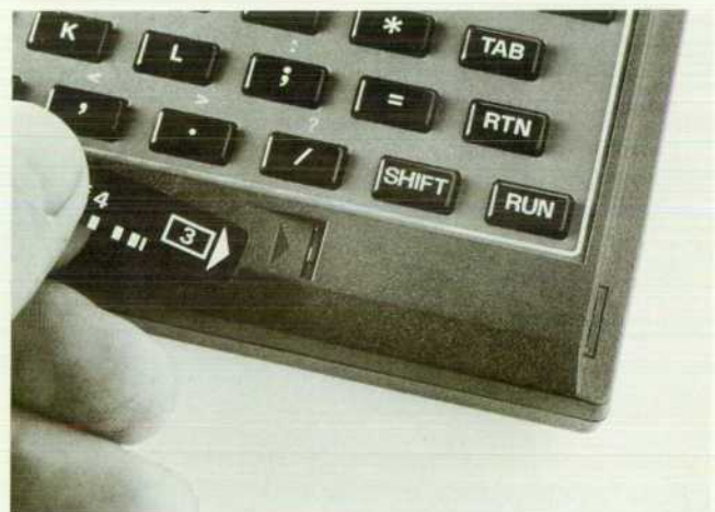
Fig. 1. The HP-75 Portable Computer's internal mass storage system uses a handpulled magnetic card reader and recorder. This unit is located in the lower right corner of the HP-75. Each card can store up to 1300 bytes of data.
