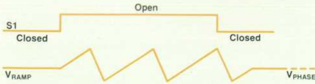
Fig. 8. Snake IC ramp generator timing in triangle mode.
