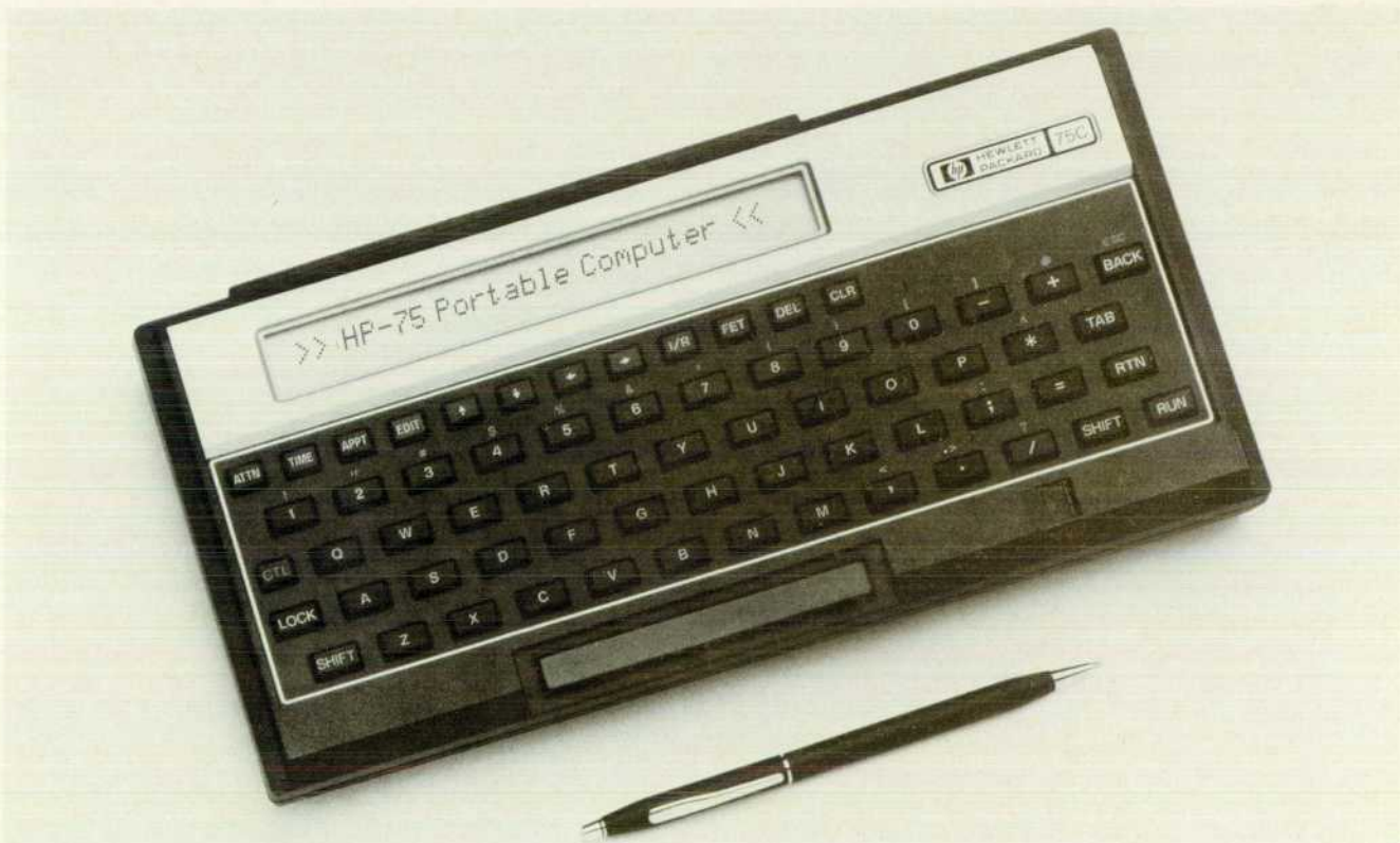
Fig. 1. The HP-75 Portable Computer is battery-powered, has a nonvolatile memory, and provides a wide variety of computational and file handling features in a small package that can be taken with you to solve problems, collect and supply information, compile reports, and even remember appointments.
