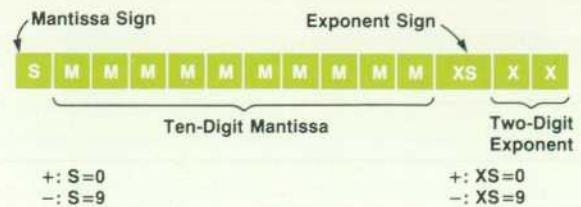
Fig. 6. The internal representation for floating-point numbers in the HP-15C uses a 14-digit (56-bit), binary-coded-decimal format.
