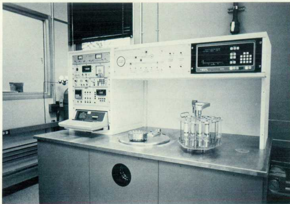
Fig. 3. Custom-designed machine bakes out, fills, and seals laser tubes.
