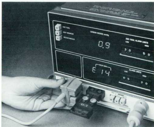
Fig. 16. The calibration stick supplied with the 47210A contains two cells that have reference concentrations of gas sealed in them. The sensor is placed on one cell at a time to check and calibrate the instrument.
