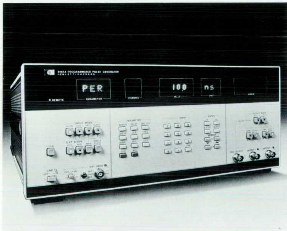
Fig. 1. Model 8161A Programmable Pulse Generator produces pulses with amplitudes up to 5V and transition times of 1.3 ns to 900 \mu s, at rates up to 100 MHz. Programming is done manually using the front-panel keyboard or remotely via the HP-IB (IEEE 488).
