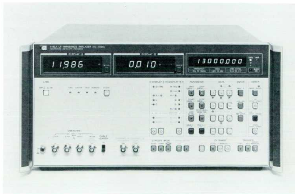
Fig. 1. The 4192A LF Impedance Analyzer makes accurate measurements of impedance and gain-phase response for components, materials, and two-port devices in the frequency range of 5 Hz to 13 MHz. Test signal levels are programmable. The analyzer has frequency-sweep capability, 4½-digit resolution, built-in dc bias that can be swept, and X-Y recorder outputs.
