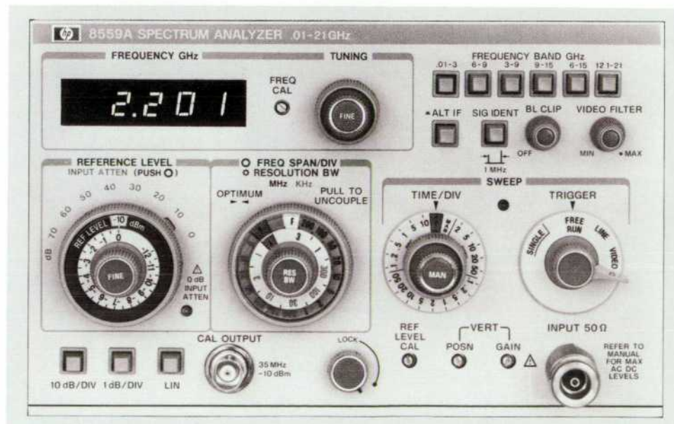
Fig. 3. The concentric INPUT ATTENUATOR and REFERENCE LEVEL (IF gain) controls are coupled such that the signal level at the reference line on the CRT, usually the top graticule line, is read directly on the REFERENCE LINE control. The concentric FREQ SPAN/DIV and RESOLUTION BW controls also move together and automatically set the appropriate sweep time (TIME/DIV). Any of these controls can be operated individually for special situations.
