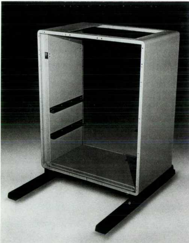
Fig. 5. The HP 300's skin serves as both cover and structure. This "minirack" is the original part and everything else is attached to it.
