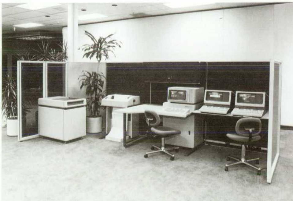
Fig. 1. An HP 300 Computer System including the system unit (center), a printer, two application terminals, and an additional disc drive. Up to 16 terminals, two printers, and 260 megabytes of disc storage can be supported by one system unit.
