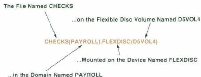
Fig. 1. A fully qualified HP 300 filename. In general, most parts of the name can be omitted and the system will assume default values.
