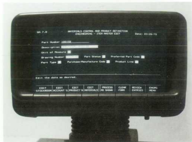
Fig. 1. Eight keys under the HP 250 CRT display can be defined differently in different applications programs to allow the operator to select various functions. The functions appear on the CRT above the keys. Also shown here is an example of a form in which data entry and display are programmed using standard INPUT, ENTER, and DISP statements.
