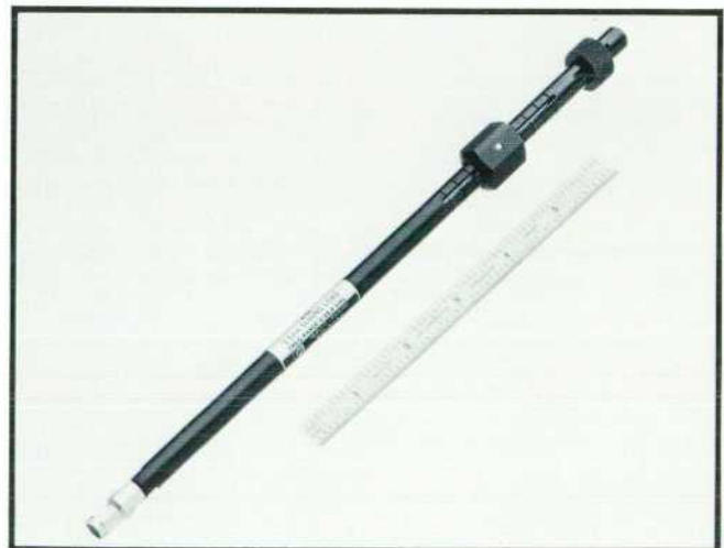
Fig. 6. Model 911C sliding load fully protects the center conductor against accidental bending. The range of the load element travel is 3/8\lambda at 2 GHz.
