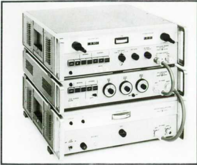
Fig. 1. System I cabinets introduced in 1961 were designed to allow the same instrument to be used either on the bench or mounted in a rack. Plastic feet fit over a cabinet below, enabling instruments to be stacked conveniently for bench use. Removal of the feet and installation of simple angle-iron brackets in the space provided enabled installation of the same instruments directly in a standard relay rack.
