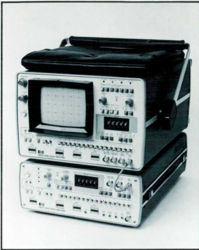
Fig. 3. Models 1600A and 1607A Logic State Analyzers work together to monitor and display 32-bit words, or work with independent clocks to examine the interaction between two digital machines. The combination of the two instruments is known as the Model 1600S. Model 1607A has most of the capabilities of Model 1600A and can work by itself using an oscilloscope or CRT monitor for the display.
