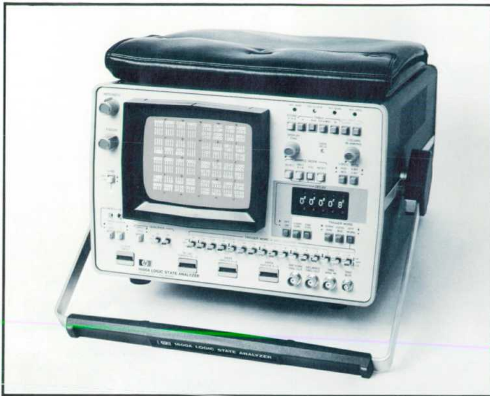
Fig. 1. Model 1600A Logic State Analyzer monitors digital data appearing on as many as 16 lines and displays the data as words of 1's and 0's in tabular form running from top to bottom on the left half of the display. The right half of the display is used for data stored in an auxiliary memory or for data acquired by a companion instrument, the Model 1607A.
