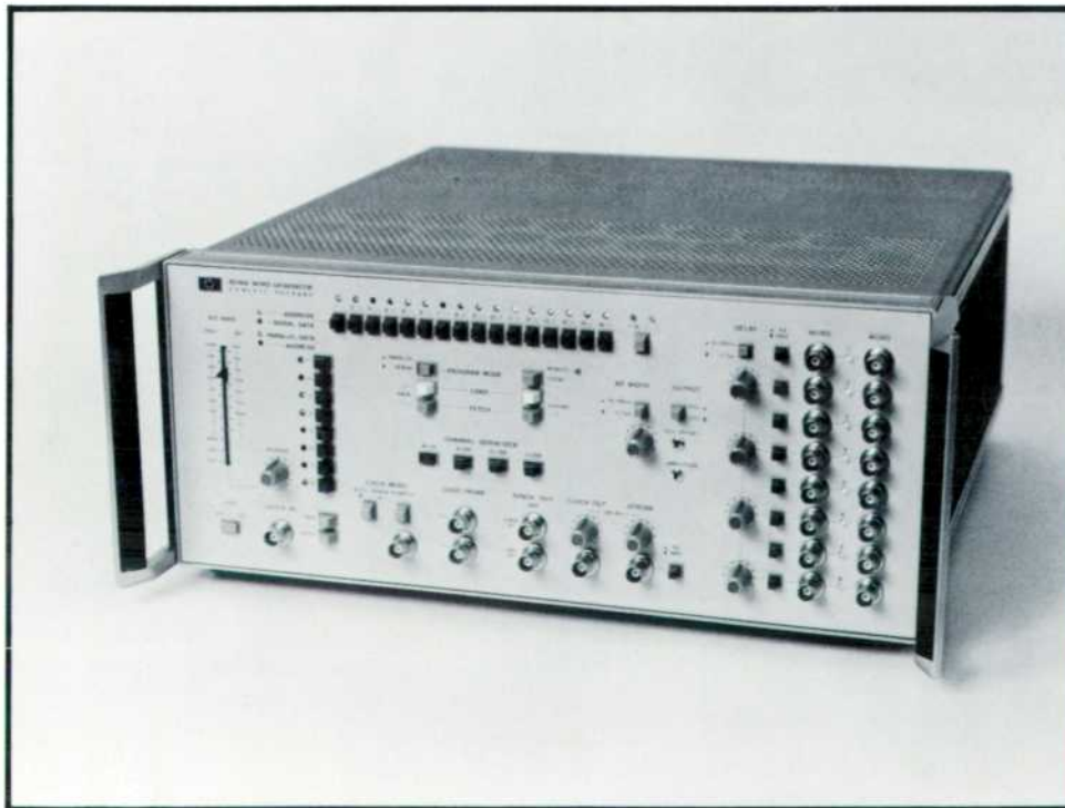
Fig. 1. Model 8016A Word Generator has eight output channels, each supplying an independently-selectable 32-bit digital word at bit rates up to 50 MHz. Operator control of the output pulse parameters broadens the range of applications for this instrument.
