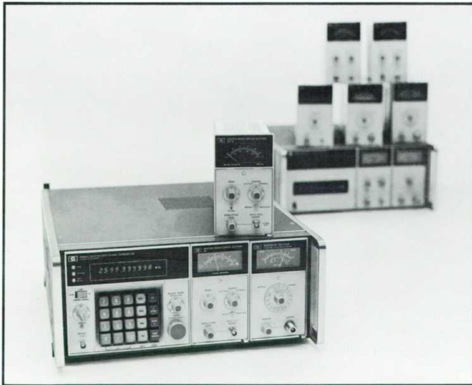
Fig. 1. The 8660-series Synthesized Signal Generator family has three new plug-ins and a new mainframe. The new RF Section plug-in gives frequency coverage to 2.6 GHz and the other two plug-ins are modulation sections that add phase modulation capability. The new mainframe and plug-ins are compatible with previously announced plug-ins and mainframes (background).
