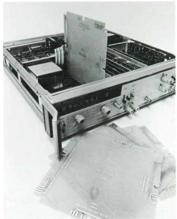
Fig. 2. Diagnostic test cards use the display to output test information, often pinpointing failures to the component level.
