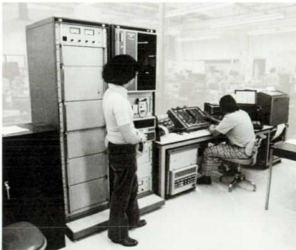
Fig. 1 Special test system completely checks 21MX CPU in ten minutes or less and troubleshoots failures to the component level 85% of the time in three minutes or less.
