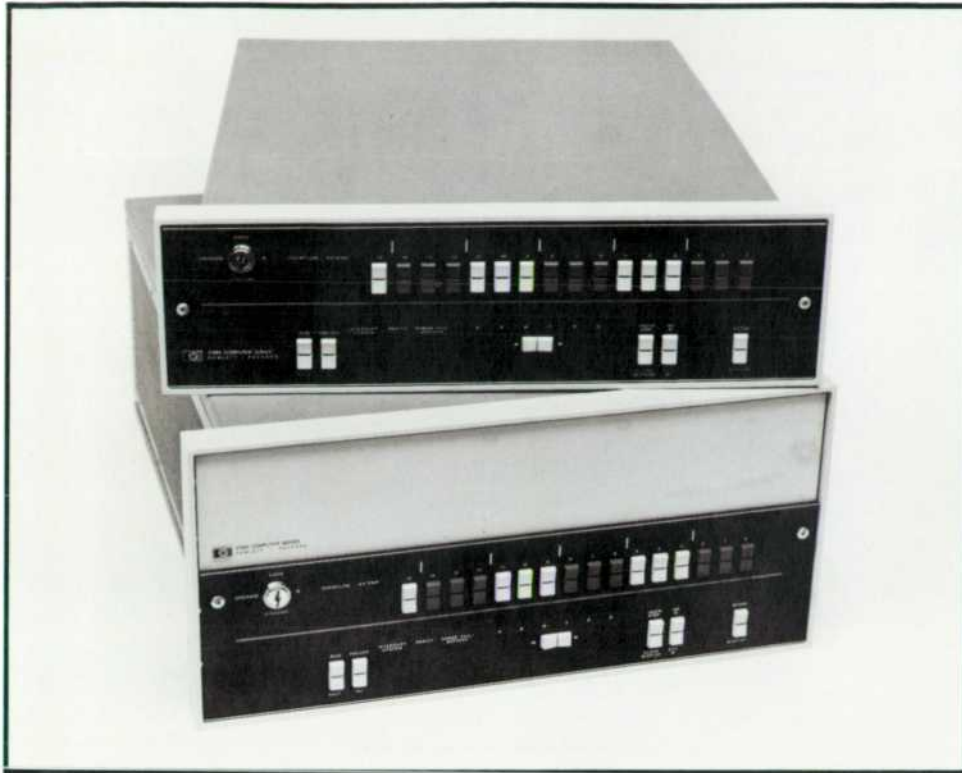
Fig. 1. The 21MX Series now consists of two computers—M110 and M120—with different levels of capability. Both are user-micro-programmable and have semiconductor main memory.
