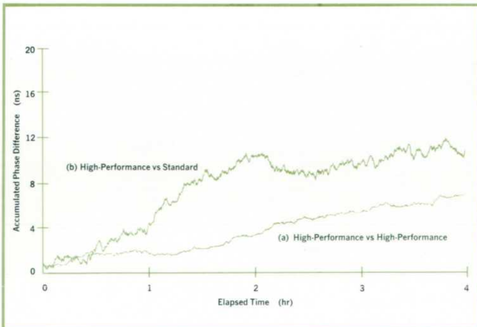
Fig. 10. Accumulated phase difference between two high-performance cesium beam frequency standards (a) and between a high-performance and a standard instrument (b). Quietness of (a) demonstrates the stability improvement of the new beam tube.
