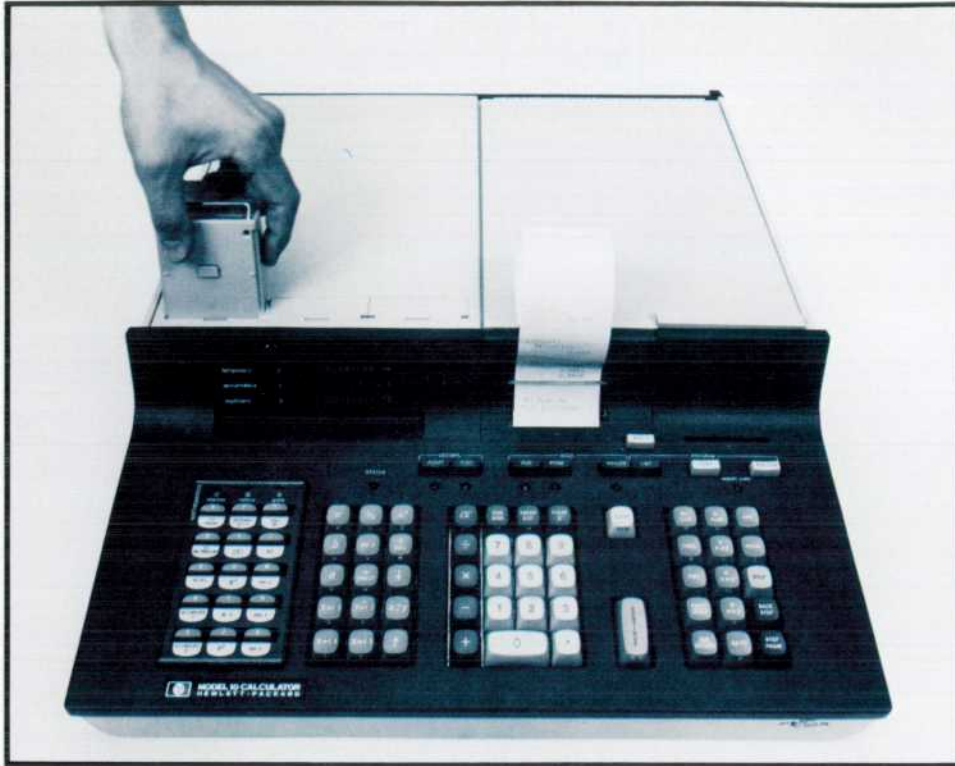
Fig. 1. Model 10 of the 9800 Series has all the capabilities of previous HP programmable calculators, plus many others. New features are the LED display, a larger internally expandable memory, decimal and indirect addressing, arithmetic operations into or from all data registers, and optional plug-in function blocks to define the lefthand keyblock and other auxiliary functions.
