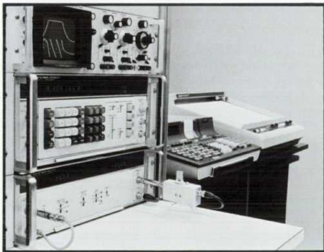
Fig. 5. Model 3042A Network Analyzer System, shown here with optional oscilloscope display and X-Y recorder, has calculator that gives Analyzer capabilities of computer-controlled system.
