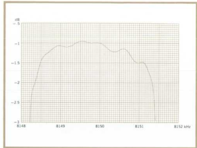
Fig. 3. Passband response of crystal filter shows detail that low residual FM of incremental frequency sweep enables in measurements on narrowband devices. Sweep had 200 frequency steps.
