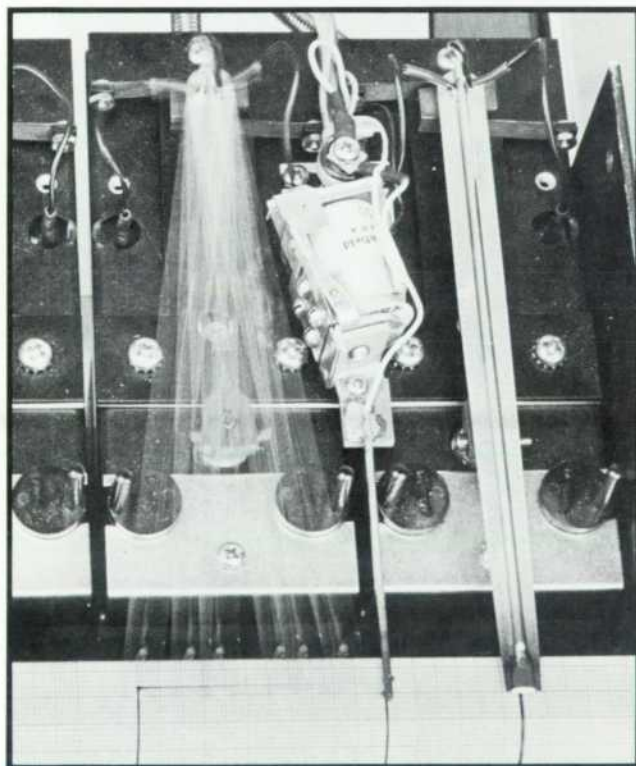
Fig. 2(b). Multiple exposure photo shows straight-line motion at galvanometer tip. (Device at center is relay operated event marker.)
