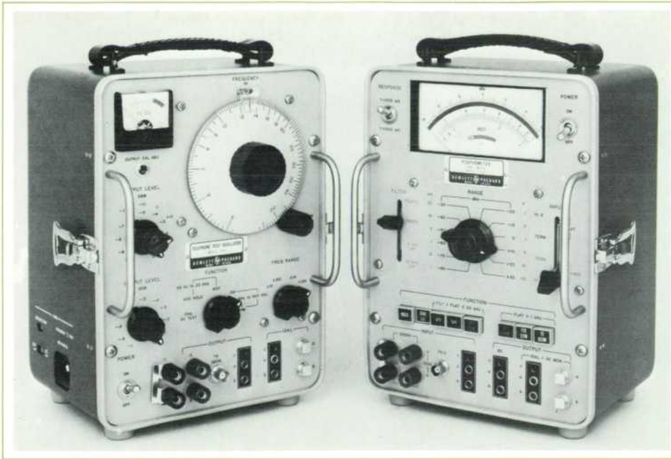
Fig. 1. The HP Model 236A Opt H10 Test Oscillator (left) and the Model 3556A Psophometer are designed specifically for making measurements on telephone systems using CCITT standards (most systems outside the United States and Canada).
