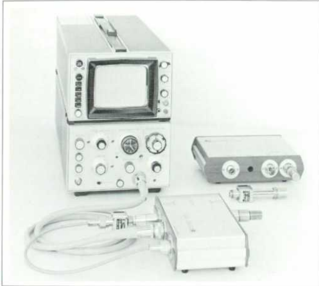
Fig. 5. 1815 Time Domain Reflectometer system works with either of two sampling heads and related tunnel-diode step generators. 1815A Plug-in here is installed in Model 181A Variable-Persistence Oscilloscope mainframe. It also works with Models 180A and 183A mainframes.
