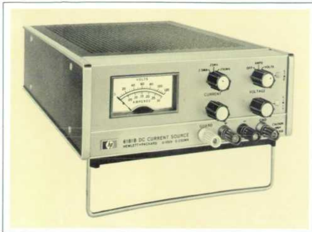
Fig. 3. New CCB Series, Models 6177B, 6181B and 6186B Current Sources, have their positive output terminals enclosed by a guard which eliminates most of the leakage currents shown in Fig. 2. They can supply currents as low as 1 \mu A, regulated within 25 ppm of setting \pm 5 ppm of range for a load voltage change from zero to maximum. They also have continuously adjustable voltage limits.
