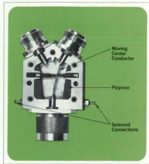
**Fig. 7.** In a slab line which has a thin center conductor (instead of a round one) the fields are extremely concentrated. This is good in a switch because it gives good isolation between output ports, and because the fields can follow the curve of the center conductor without dispersion. **Fig. 8.** Broadband (dc to 18 GHz) coaxial switches typically have insertion losses less than 0.5 dB and VSWR's less than 1.2. Isolation is greater than 50 dB at 12.4 GHz, and greater than 45 dB at 18 GHz.
