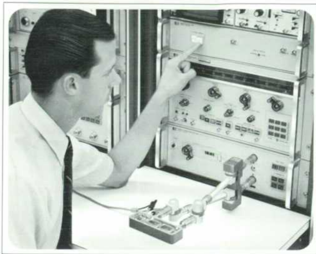
Fig. 2. The thin-film amplifier in the foreground is about to have its s -parameters measured automatically by the HP 8541A Automatic Network Analyzer, a computer-controlled system programmed in BASIC or FORTRAN. Programs for performing many tests are supplied with the system. Special tests are programmed by the user.
