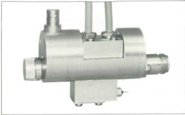
Fig. 10. Exterior view of new mixer. Diode is inside cap at left.
