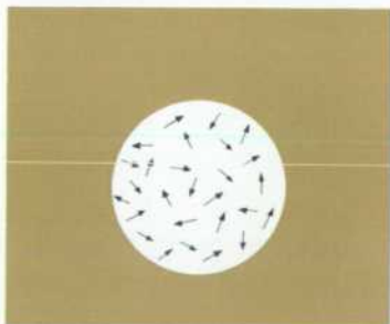
(a) Randomly oriented magnetic dipoles in the unmagnetized ferrite.
