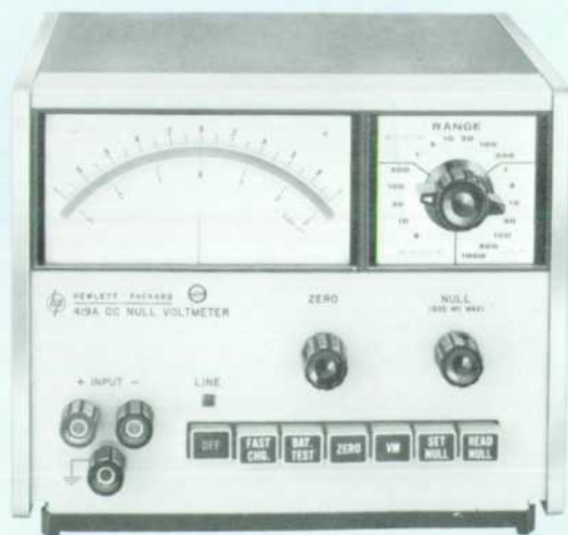
Fig. 2. -hp- Model 419A DC Null Voltmeter has 18 measuring ranges from 3 \mu\text{V} end scale to 1000 \text{ V} end scale. Pushbuttons select operating mode. Voltmeter operates from ac line power or from rechargeable internal batteries.
