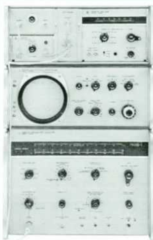
Fig. 1. New -hp- Model K15-8551B Spectrum-Analyzer Up-Converter mounted on top of -hp- Model 851B/8551B Spectrum Analyzer. Analyzer range without converter is 10 MHz to 40 GHz; converter extends this down to 10 kHz.
