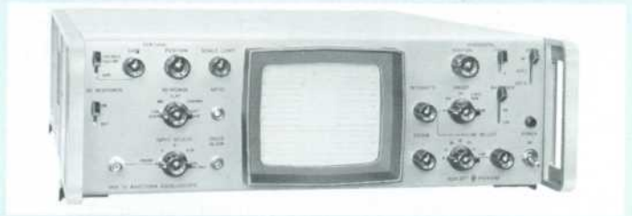
Fig. 1. New -hp- Model 191A Television Waveform Oscilloscope. Oscilloscope is specially designed to facilitate testing of color and black-and-white TV transmission lines and systems in which new VITS signals are used. Instrument is all solid-state (except CRT).
