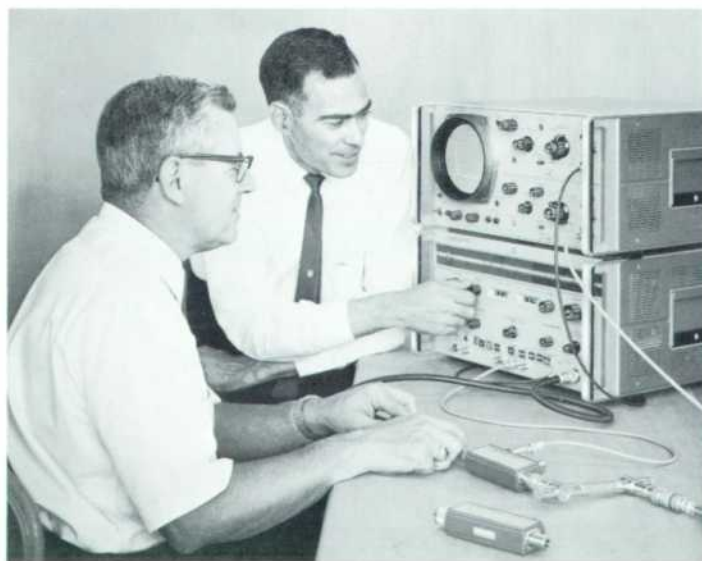
Fig. 1. Flat frequency response of new -hp- Directional Couplers and Detectors is especially advantageous in closed-loop power-leveling systems, such as in the swept-frequency evaluation of coaxial filter frequency response being made here by -hp- design engineers Larry Renihan (left) and Auber Ryals. Directional Detector, which supplies error signal for automatic leveling loop, senses RF power right at point of measurement.
