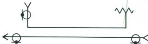
Fig. 2. Coaxial Directional Coupler -hp- Model 796D, shown at left and in schematic form above, has high directivity, insertion loss of only about \frac{1}{4} db, and SWR of 1.15 throughout range of 960 to 2110 Mc. Model 797D is for frequency range of 1900 to 4100 Mc and 798C is for 3.7 to 8.3 Gc.
