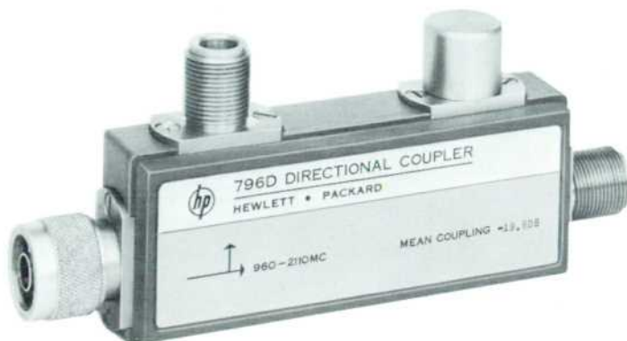
Fig. 2. Coaxial Directional Coupler -hp- Model 796D, shown at left and in schematic form above, has high directivity, insertion loss of only about \frac{1}{4} db, and SWR of 1.15 throughout range of 960 to 2110 Mc. Model 797D is for frequency range of 1900 to 4100 Mc and 798C is for 3.7 to 8.3 Gc.
