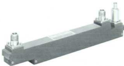
Fig. 12. Directional Detectors for X-band consist of three waveguide sections with coupling holes between both interfaces. Coupling to bottom section "drains" enough energy to flatten frequency response of directional coupler formed by top and center sections.
