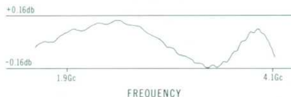
Fig. 6. Frequency response of typical 787D Directional Detector.
