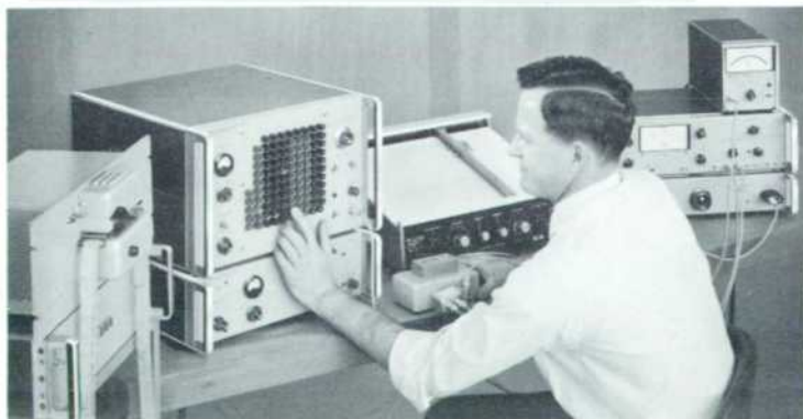
Fig. 1. New hp Model 5100A/5110A Frequency Synthesizer generates high-stability signals in 0.01 cps increments from dc to 50 megacycles. Generated frequency can be controlled by panel keyboard or by remote control. Programmed control tapes can be used to specify frequency patterns for automatic testing, fast receiver tuning, NMR work, etc.
