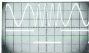
(a) (Upper trace) Synthesizer frequency switched from 20.003 Mc to 20.006 Mc and back with 20 Mc subtracted to display switching in greater detail. This switching detail is typical of any of the six right-hand places. Sweep speed is 200 \mu\text{sec}/\text{cm} .
