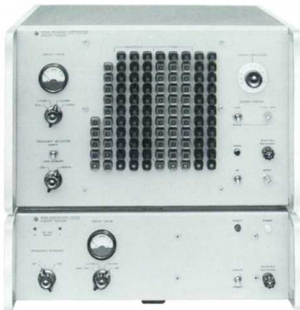
Fig. 3. -hp- Model 5100A Synthesizer (upper unit) with Model 5110A Synthesizer Driver (lower unit). One Driver unit can operate up to four Synthesizer units.
