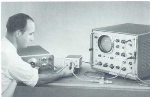
Fig. 1. New broadband, solid-state amplifier is built in two versions. Model 462A Pulse Amplifier, shown here, has frequency response characteristics optimized for best transient response. Model 461A has flat frequency response that places -3 db points at 1 kc and 150 Mc.
