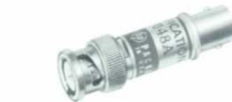
Fig. 7. Accessory feed-through termination has built-in 50-ohm resistance for terminating amplifier output while providing an output connection for external high impedance circuits.
