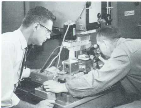
Fig. 5. Air-bearing spindle mounted on drill head of tape-controlled machine tool. Drill head serves only as fixed mount since spindle has own motor and enclosed belt drive for minimum vibration. Operator, looking at work piece, requires microscope because of small dimensions. In this application, work piece is raised by small, cam-driven table guided by flat air-bearings to achieve extremely smooth movement.
