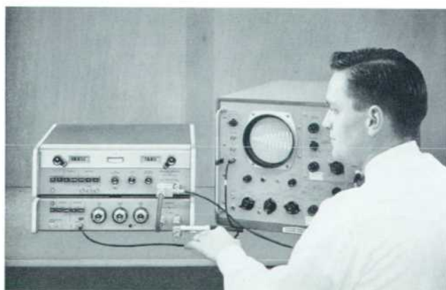
Fig. 1. New -hp- Model 8714A Modulator gives wide versatility in modulating waves in the 0.8–2.4 Gc range and greatly reduces incidental FM and other effects. Trace on scope shows build-up of 1 Gc RF pulse, is described further on p. 4.
