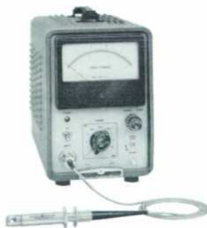
Fig. 3. Probe operates in conjunction with -hp- 428B Milliammeter.
