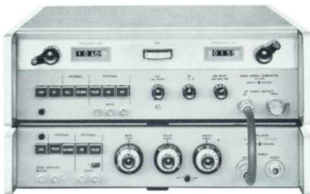
Fig. 10. -hp- 8714A Modulator (lower unit) shown with new -hp- 8614A 0.8-2.4 Gc Signal Generator to be described in future issue.
