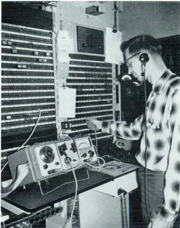
Fig. 2 (at left). -hp- 3550A Portable Test Set measures insertion loss and frequency response of telephone lines over range from 50 cps to 560 kc. Unit matches 135, 600, and 900-ohm lines, is transistorized and battery-operated.
