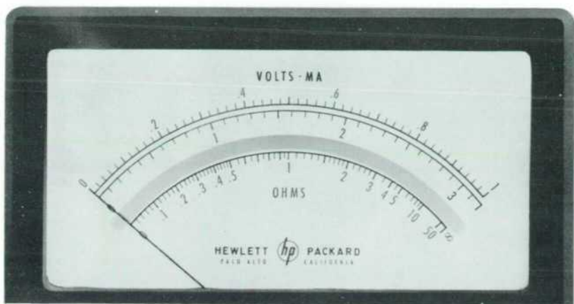
Fig. 6. Three-quarter size reproduction of meter face used on new voltmeter. Meter movement itself has very large torque-to-weight ratio to virtually eliminate frictional effects.
