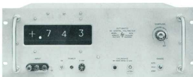
Fig. 1. New -hp- digital dc voltmeter has been designed as a fully automatic instrument for measuring voltages from 1 millivolt to 999 volts of either polarity. Coded outputs are provided for automatic data logging in conjunction with -hp- digital recorder or for driving other data handling equipment. Readout system includes a window of light-polarizing material which virtually eliminates effect of external light and gives a very dark, soft background of maximum contrast for ease in reading.
