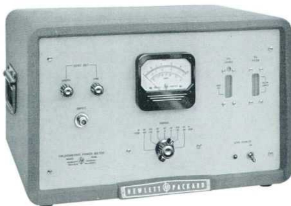
Fig. 1. New -hp- Model 434A Calorimetric Power Meter measures powers between a few milliwatts and 10 watts at frequencies from dc to 12.4 kilomegacycles. Self-balancing type circuitry makes operation automatic and gives reading in less than 5 seconds. Instrument is provided with 50-ohm coaxial input.
