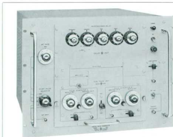
Fig. 1. New hp Model 218A Digital Delay Generator produces output pulses after digitally adjustable precision intervals of up to 10,000 microseconds on command of external signal to simplify calibrating and testing systems where time interval or delay time is important. Instrument can also count and produce outputs after any de-
