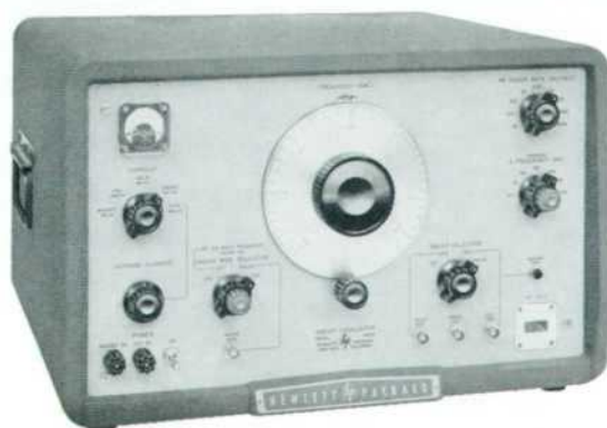
Fig. 1. Besides providing c-w, a-m, and f-m outputs, -hp- Model 686A voltage-tuned oscillator sweeps over full 8.2 - 12.4 kmc range or increments as small as 4.4 mc. Wide range of sweep rates enables measurements to be plotted on recorder or displayed without flicker on oscilloscope. Manual trigger facilitates permanent recording.
