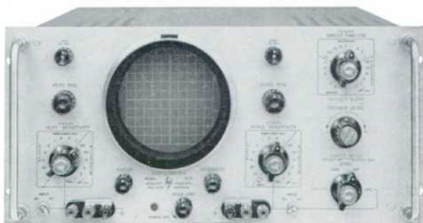
Fig. 1. New hp -Model 130BR DC-300 KC Oscilloscope is designed with high sensitivity, high stability, wide range of sweep speeds, x5 expandable sweep, and identical amplifiers so as to simplify measurements of voltage, time and phase shift. Console operation is facilitated by additional input terminals at rear of chassis.
