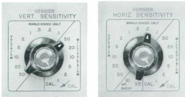
Fig. 6. Vertical and horizontal sensitivity controls are simple, direct-reading type which are identical except for x1 and x5 sweep positions at ccw end of horizontal control.
