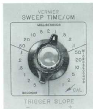
Fig. 4. To simplify sweep selection, sweep time selector is a single, direct-reading control. Concentric vernier enables continuous variation between steps.
