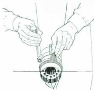
Fig. 8. Crt alignment lever simplifies angular tube positioning.
