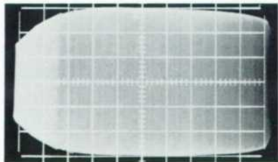
Fig. 1. Oscillogram of response of quality matching transformer at -30 dbm made by observing transformer output directly on oscilloscope while driving transformer and its amplifier from new -hp- single-band audio oscillator.
