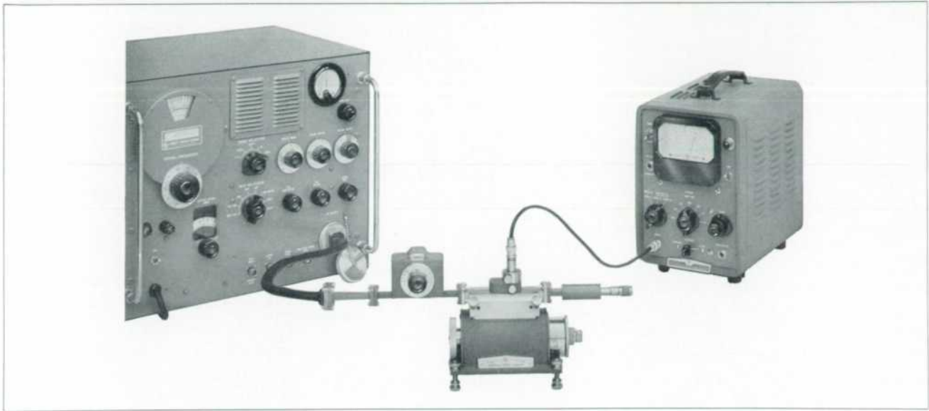
Fig. 5. New slotted line equipment used with -hp- 415B Standing Wave Indicator and 628A SHF Signal Generator.
