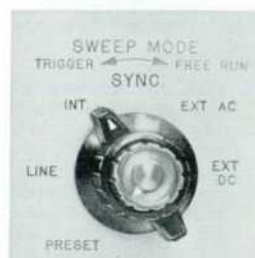
Fig. 8. Trigger Level and Slope controls (above) with Sync and Sweep Mode controls (below). When Sweep Mode control is in Preset position, sweep triggers automatically on most waveforms.
