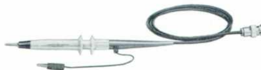
Fig. 2. Probes for new oscilloscope have slim easy-to-use shape and flange-operated alligator clips. Probe capacity can be adjusted without tools merely by loosening finger-operated nut at right of second flange. See description on p. 5.
