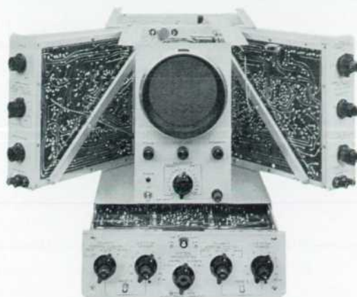
Fig. 13. Model 150A has been designed to afford high degree of accessibility to parts as indicated by above view of instrument with cabinet removed.
