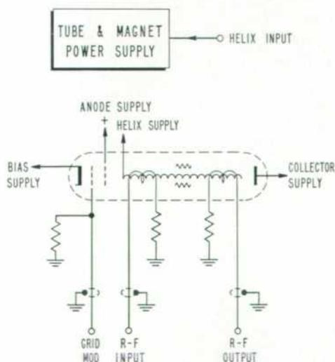
Fig. 2. Basic circuit arrangement of new amplifiers.
