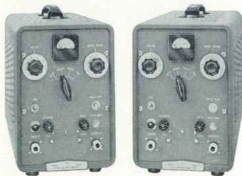
Fig. 1. New -hp- 492A and 494A Traveling-Wave Tube Amplifiers give more than 25 db of gain over 4-8 and 7-12.4 kmc ranges. Special modulation provision enable the amplifiers to be used to simulate doppler effects, to obtain amplitude-modulated signals or to form high-sensitivity linear detectors.
