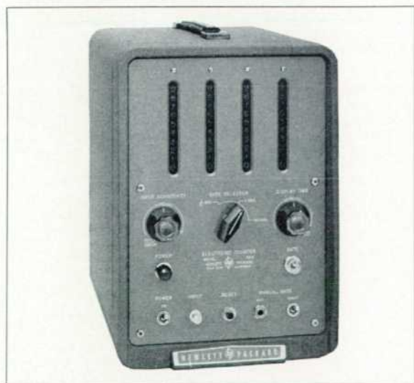
Fig. 1. New -hp- Model 521A Industrial Electronic Counter measures frequencies up to 120,000 cycles per second. Internal time base system can be operated from power line frequency, from optional precision oscillator, or from existing standard frequencies.
