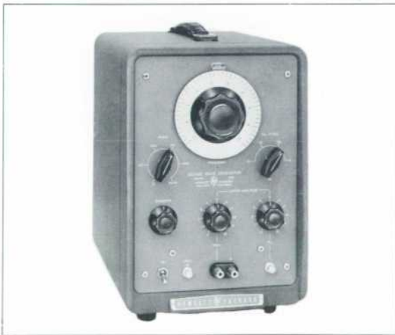
Fig. 1. New hp -Model 211A Square Wave Generator operates from 1 cps to 1 megacycle, has only 20 millimicroseconds rise time from fast output. A second output provides up to 55 volts peak-to-peak.
