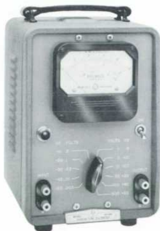
Fig. 1. New hp Model 400AB operates from 10 cps to 600 kc, is accurate within 3%. Voltages as low as 0.3 millivolt can be measured. Output terminals permit use as high-gain amplifier. Collapsible bail on bottom permits meter to be tilted.
