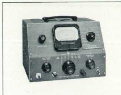
Fig. 7. -bp- Model 430B power meter as modified for use with Model 477A coaxial thermistor mount. New bias current switch is at upper right of panel.
