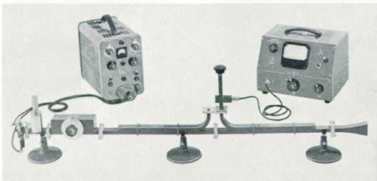
Fig. 1. Two -hp- multi-hole directional couplers in a reflectometer arrangement for measuring reflection coefficient magnitude. In background are an -hp- 715A klystron power supply to power signal source and an -hp- 415A standing-wave indicator to read output of detector.
