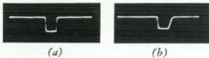
Fig. 2. Oscilloscope waveforms of typical 1 microsecond r-f pulses (rectified) generated by (a) Model 614A and (b) Model 616A.
