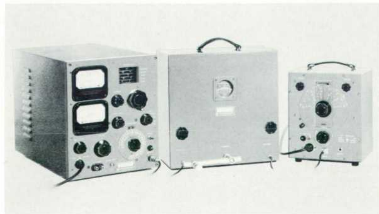
Figure 1. -hp- Model 608A VHF Signal Generator Used with New -hp- Models 803A VHF Bridge and 417A VHF Detector.
