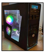
Will Pitts proudly presented his new build. This is a modern Windows 11 computer based on the Gigabyte GA-H57M-USB 3.0 motherboard, equipped with a Core i7 870, 8GB RAM, 128GB SSD and a 1TB hard drive. This motherboard has the unique ability to support one floppy, so Will decided to incorporate a 5.25" drive. His objective, years in the making, was to have a modern build with a 5.25" floppy drive. Congratulations to Will! He mentions that his next project is connecting an 8" floppy drive.
