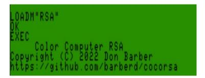
Don Barber shared "Color Computer RSA", a software piece that he wrote. He states, "This is a program for the Tandy / Radio-Shack TRS-80 Color Computer to perform RSA key generation, encryption, and decryption. The code is all written in 6809 assembly. It will operate with up to 2048-bit keys." The software, along with its source, is available at the following link:
